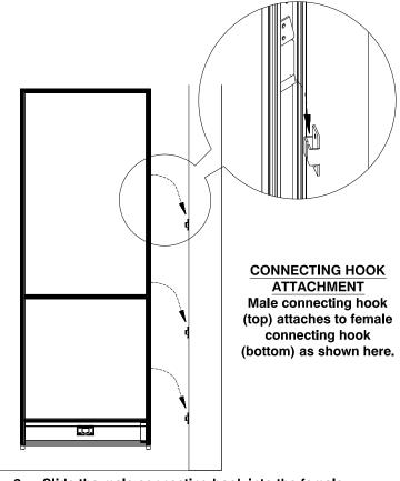
Slide the male connecting hook into the female connecting hook to secure panel to wall. See hook attachment detail.
